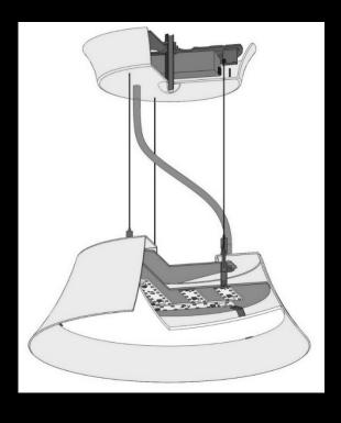
spun aluminum canopy painted to match fixture holds three ultra-thin vertical stainless steel cables with field adjustable micro-grippers for exact AFF mounting height
